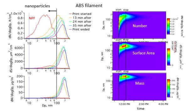
3D Printer Particle Emissions: Size distribution evolution with printing time, evolve from small to larger particles
