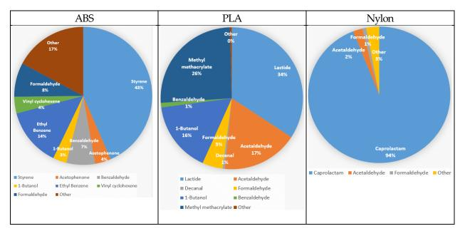
Comparison of VOCs from 3D Printers by Filaments during Operation
